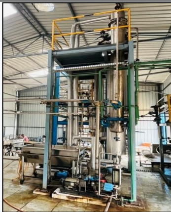
Multiple Effect Evaporator for Jaggery Processing
