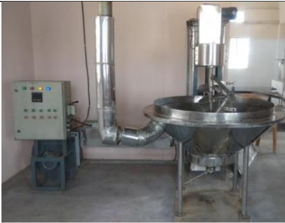
Hot jaggery stirring and filling mechanism
