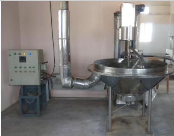
Hot jaggery stirring and filling mechanism
